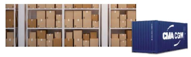
**Definition:** A freight container, totally enclosed and weatherproof, with a rigid roof, rigid side walls, and floor, having at least one of its end walls equipped with doors and intended to be suitable for the transport of a variety of cargoes.
